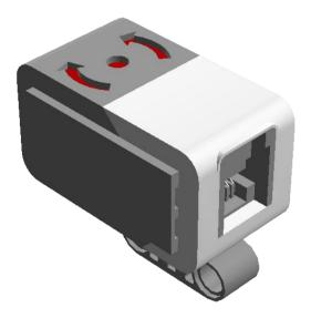
First must correct for sensor *bias* and *drift* sometimes shows movement even when still
